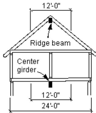
**Figure 5 - This figure illustrates 2 structural elements: a structural ridge beam and a center girder. Both have a tributary area of 12'0". The load per foot of beam is determined the same way as for headers.**
